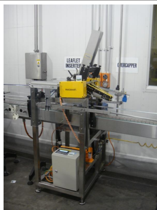
The PF400 with stand, glue system and guarding
